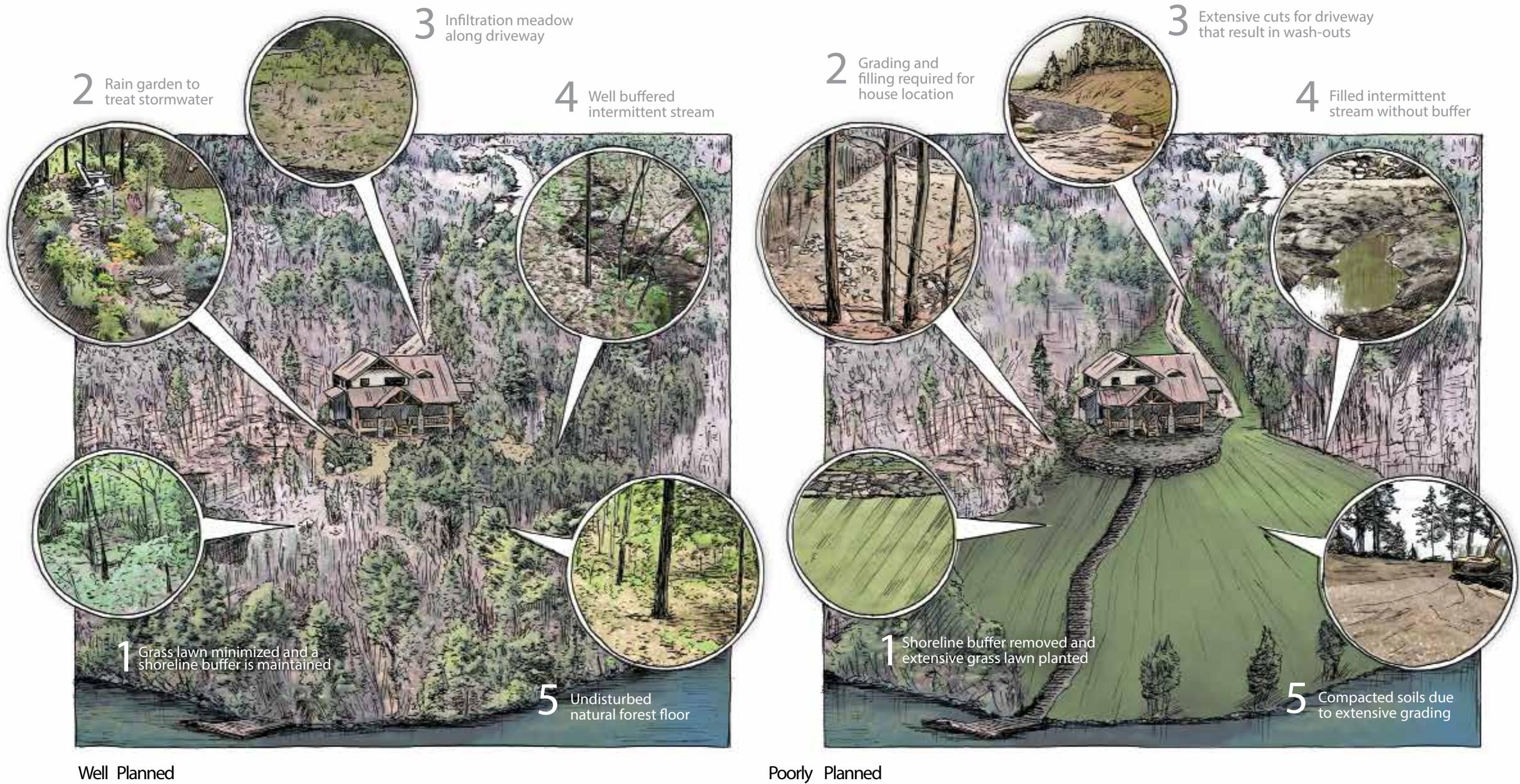
FIGURE 6: The Importance of Maintaining Natural Drainage Patterns When Developing a Property
