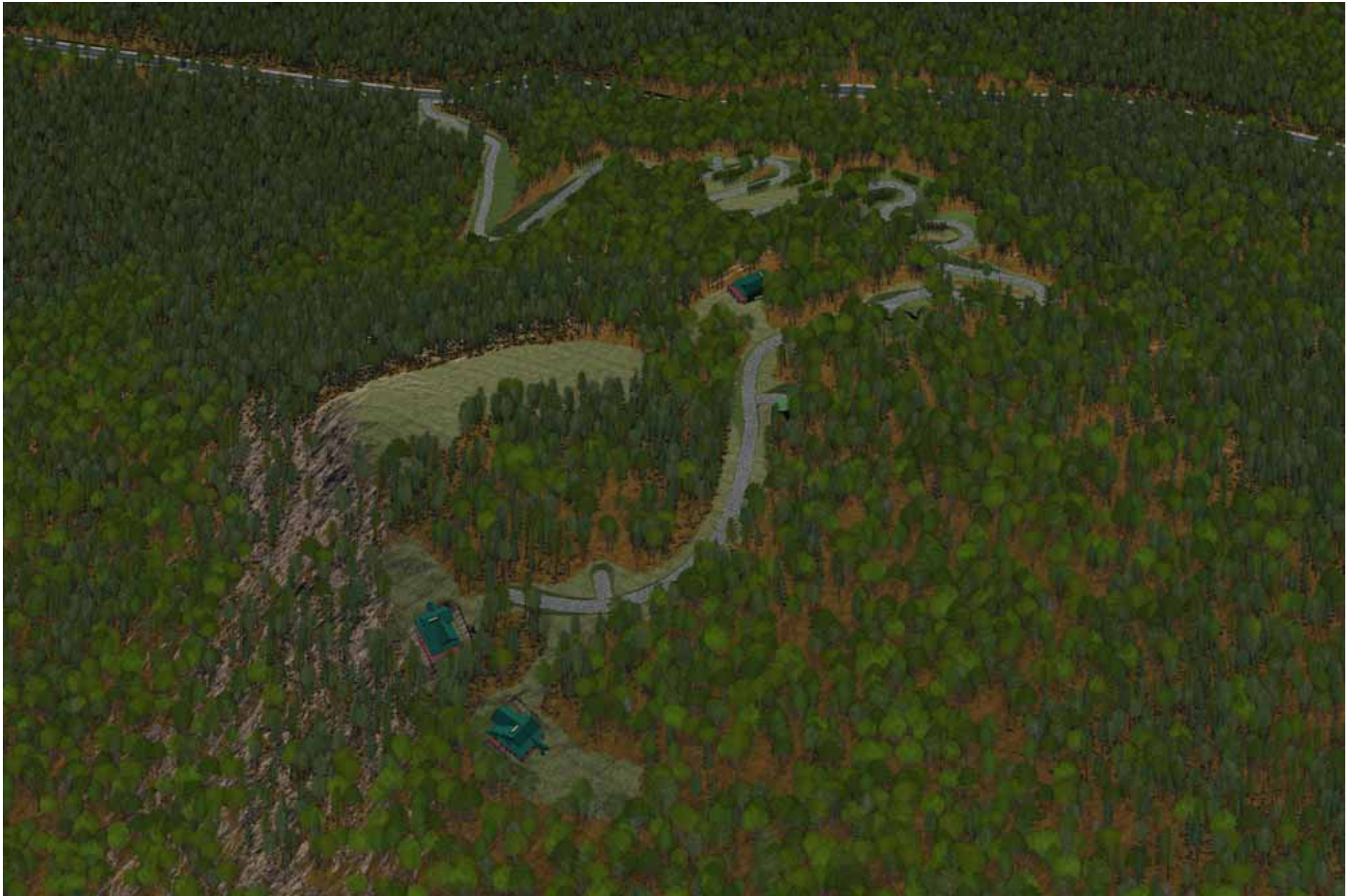
Access Road Viewed From Helicopter Partial Revegetation--Leaf On
